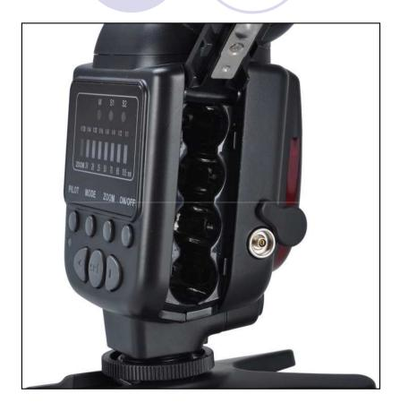
MG-68 includes PC sync port which enables the flash at the camera's maximun flash sync speed if triggered by the Trigmaster.
