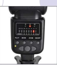
MG-68 can work as an offcamera auxiliary flash. When the master flash fires even the first time, it will trigger MG-68 flash directly.
