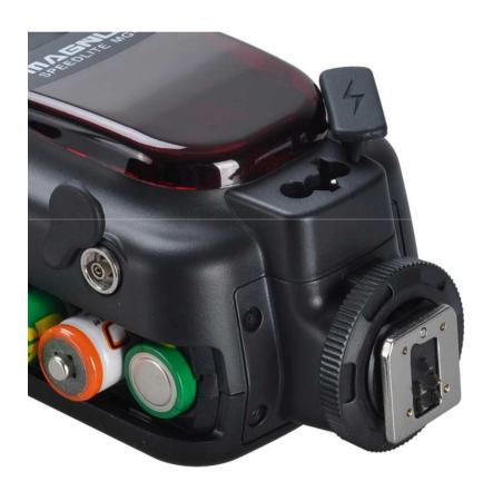
MG-68TL includes PC sync port which enables the flash at the camera's maximun flash sync speed if triggered by the Trigmaster.
