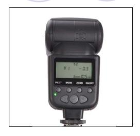
MG-68TL can also work as an off-camera auxilliary flash while shooting your master flash in TTL mode. MG-68TL will ignore the pre-flash of the master flash. While the master flash fires, it will trigger MG-68TL.
