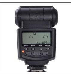
MG-58TL can work as an off-camera auxiliary flash. When the master flash fires even the first time, it will trigger MG-58TL flash directly.
